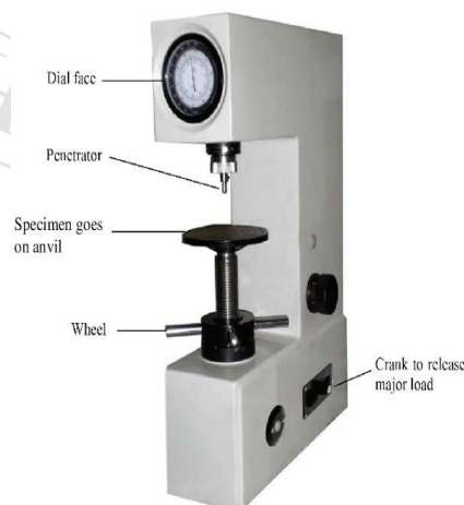
Figure 14.1 : Rockwell Hardness apparatus.
