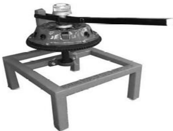
Fig..3.9 Working Model of Single Plate Clutch Fig. 3.10 Multi-plate Clutch Assembly
