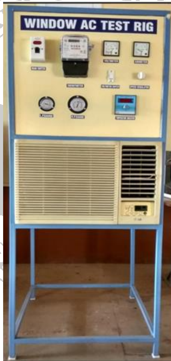
Figure 7.1: Window air conditioner test rig
