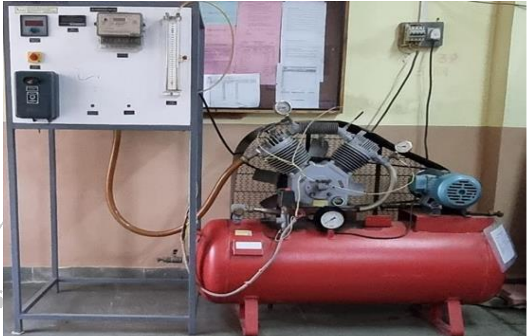
Figure 18.1 - Set up of two-stage reciprocating air compressor
