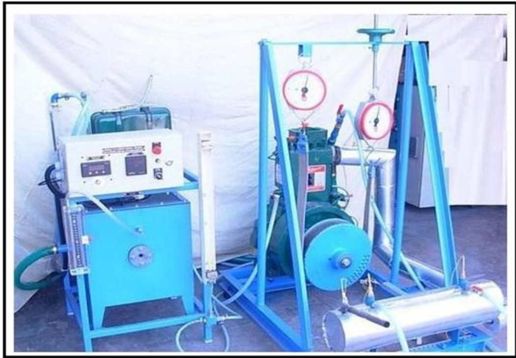
Figure 11.2 - Four-stroke engine test rig with rope brake dynamometer
