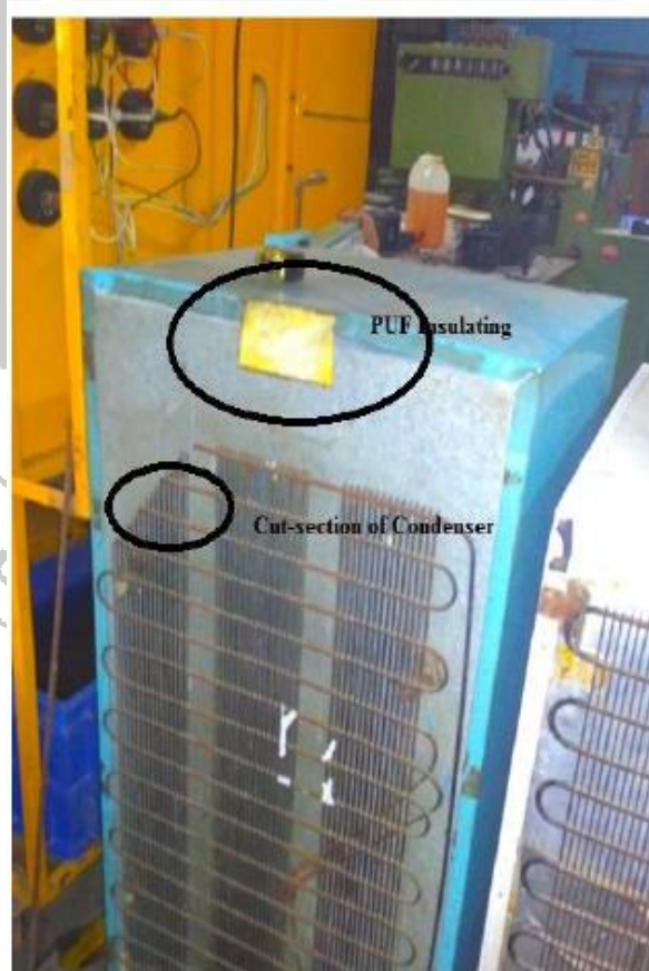
Figure 1.3 Actual Cut-section of household refrigerator representing PUF insulating back panel, Condenser coil.
