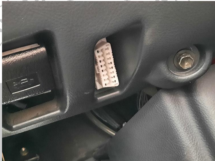
Figure 15.2 – Location of ECU port for OBD II Scanner connection
