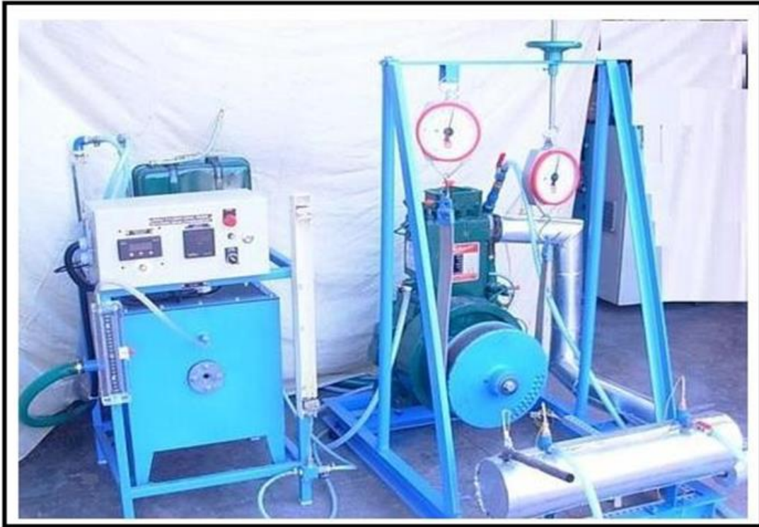
Figure 9.4 - Four-stroke engine test rig with rope brake dynamometer
