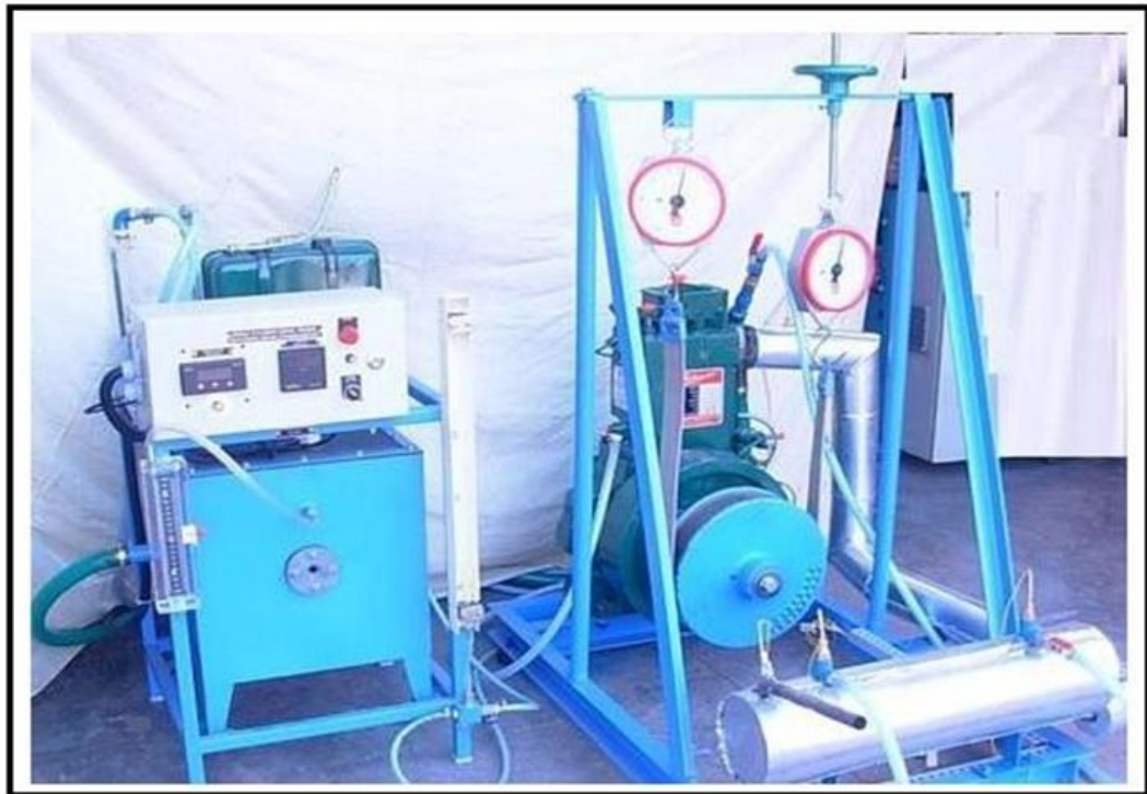
Figure 10.4 - Four-stroke engine test rig with rope brake dynamometer
