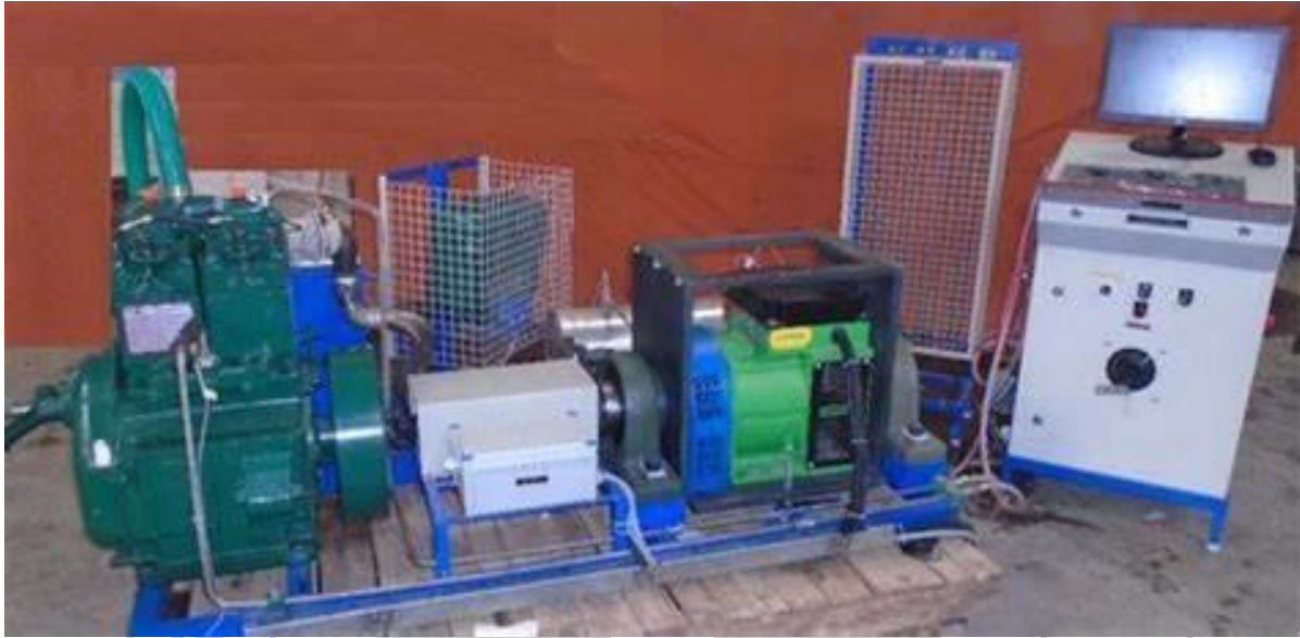
Figure 12.3 Four-stroke Four-cylinder Petrol engine Morse Test rig
