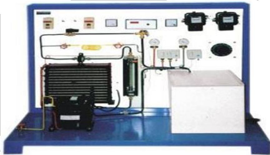
Figure 2.1 Vapor compression refrigeration Test rig
